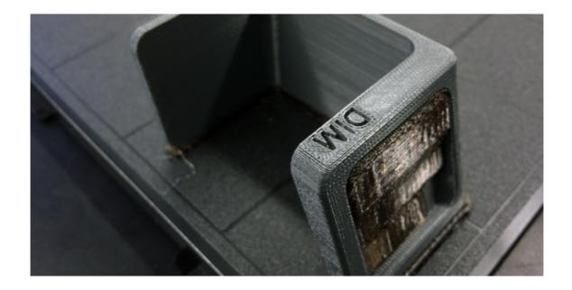
There are, however, clear stepping lines between the printed layers. If we don't remove these stepping lines, they'll show up in the final paint coat which will ruin our smooth finish. Thankfully, removing these will be easy thanks to ABS's high melting point and easy sandability.
