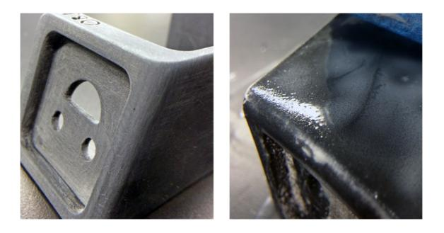
*Left:* Removing the residue will reveal a harder surface that we can paint on. *Right:* Wet sanding through 600 grit to remove the residual layer is very effective, thanks to the Objet's water soluble support material.
