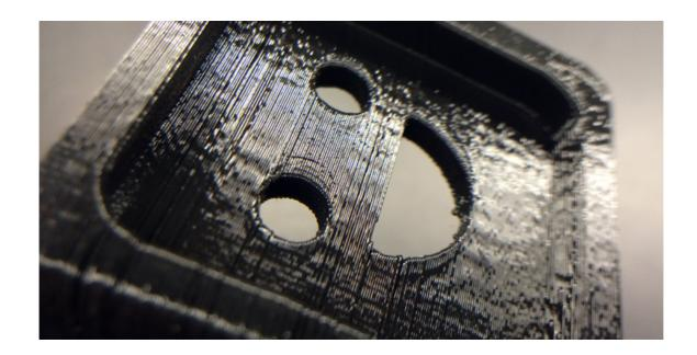
A PLA print from a 5th generation Replicator. Notice the severe stepping between layers and the unevenness of layers in the plane of the print.
