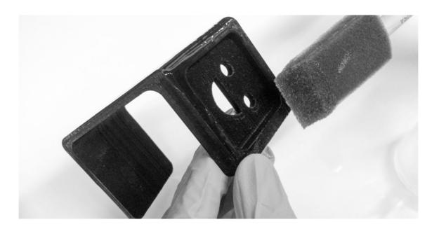
Applying a thin (1/64") coat of XTC-3D. Watch out for areas where XTC-3D may pool up, such as internal pockets.
