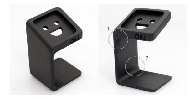
A finished VeroBlack part. **Circle 1:** Notice how areas where the residue was not properly removed have a powdery paint finish. **Circle 2:** Faint stepping is visible in the paint finish, but for the most part starting with a smooth part has resulted in a smooth paint finish.
