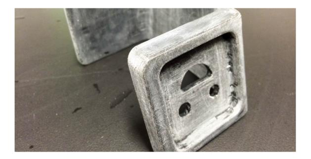
Sanded and cleaned PLA part that has been coated with XTC-3D. Notice how the internal pockets have pooling and are also poorly sanded.
