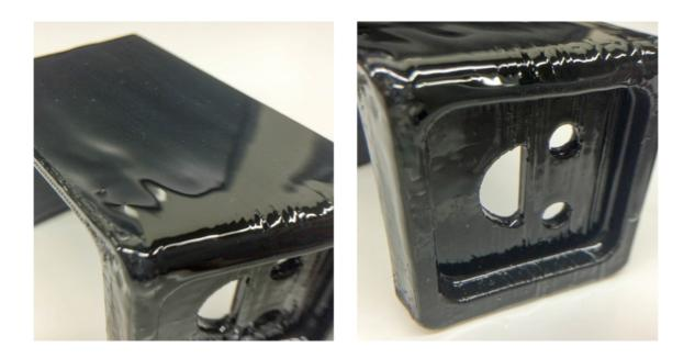
*Left:* A thin coat of XTC-3D. Notice how striations are still visible in the reflection of the part. Multiple coats may be needed to achieve a flat surface. *Right:* Apply thin coats to avoid pooling in internal pockets.
