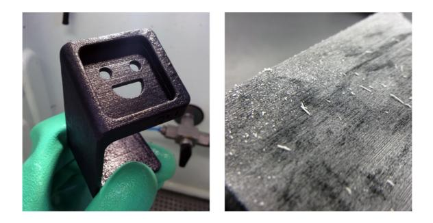
*Left:* freshly cleaned VeroBlack part out of bath after support material removal. *Right:* After drying there will still be trace amounts of residue which will fall off in small soft white chunks with dry sanding at around 100 to 300 grit. The Objet30 prints come out of the printer with a thick layer of support material so before we can begin finishing our VeroBlack part, we'll need to remove this support and the residue it leaves behind.
